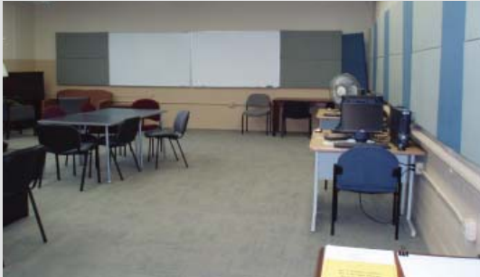
Above: The cozy new lounge area at Cardozo Senior High's PCRC Below: The central multi-use space now has acoustical panels to improve the quality of sound within
